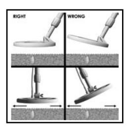
Figure 5. "sweeping" the search coil. Keep the search coil parallel and close to the around at all times
